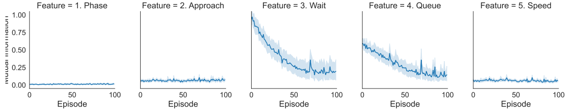
Figure 4-8: Evolution of the mutual information between the reward and each of the five features considered in the RESCO benchmark for Traffic Signal Control during learning in the 21-intersection use case. The mean and 95% CI across 21 intersections are shown.
