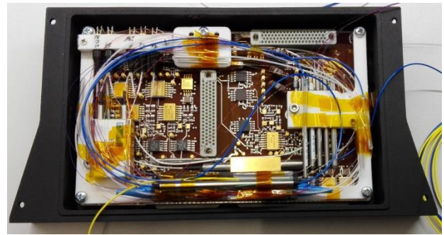
Figure 6. AFE Electronics board with first version of the OFE design integrated in the mechanical AFE frame.
