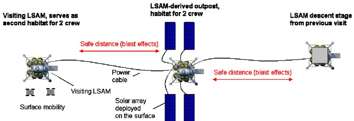
**Figure 7: Intermediate outpost configuration on the lunar surface. Middle LSAM lander is pre-deployed uncrewed and carries consumables and equipment instead of ascent propulsion. LSAM lander to the left is a visiting LSAM that brings the crew and serves as habitat for 2 crewmembers during the surface stay. Landers are connected by cable; re-supply of the visiting LSAM is achieved using the surface mobility assets.**
