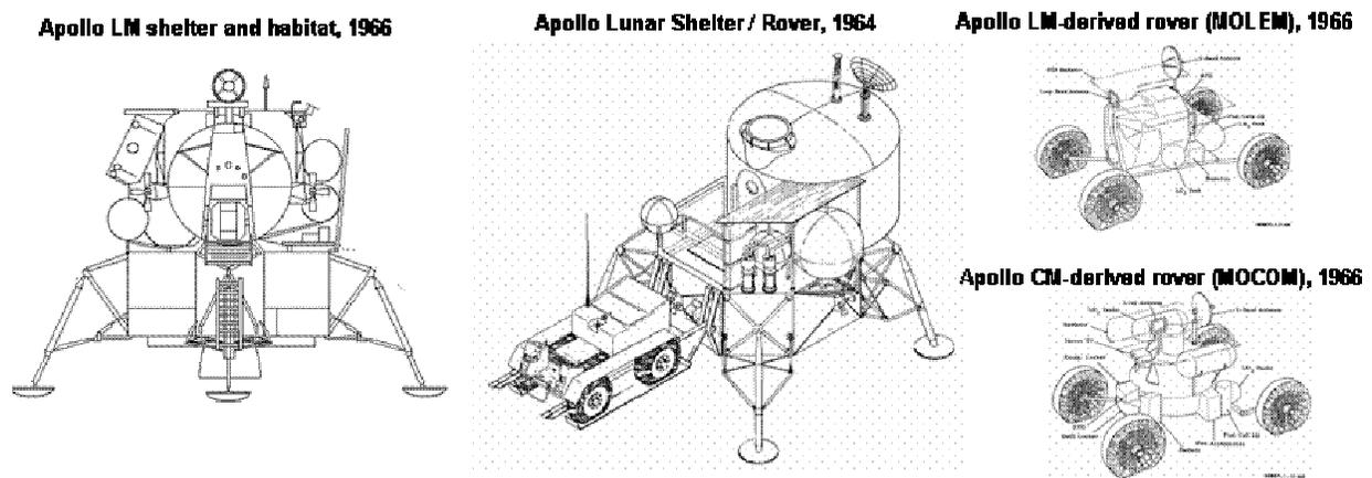
**Figure 1: Lunar surface operations hardware concepts designed for the Apollo Applications Program (AAP); all concepts use elements derived from the Apollo lunar sortie hardware.**
