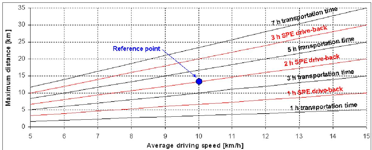
**Figure 2: Maximum straight-line distance from outpost (Moon / Mars) for a traverse configuration involving two pressurized vehicles. Black lines represent different times available for transportation along the traverse and red lines represent different drive-back time requirements in case of a Solar Particle Event (SPE). The reference point is based on the assumption that the crew has to be back at the outpost 2 hours after information of the SPE has been received.**
