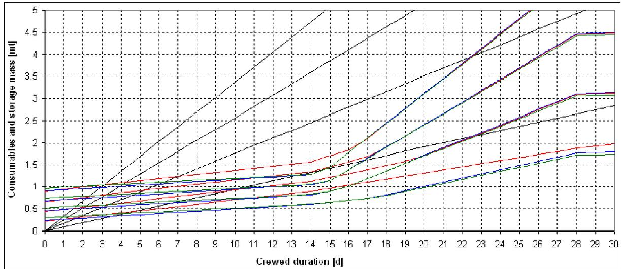
**Figure 14: Mass requirements for extended polar LSAM stays of 2 crewmembers. Black lines represent baseline configuration (fuel cells, LiOH, no regeneration), red lines represent baseline configuration plus solar panels, blue lines represent red configuration plus wash water regeneration, green lines represent blue configuration plus regenerative CO<sub>2</sub> removal. Contours represent different power levels, highest 20 kW, lowest 5 kW.**
