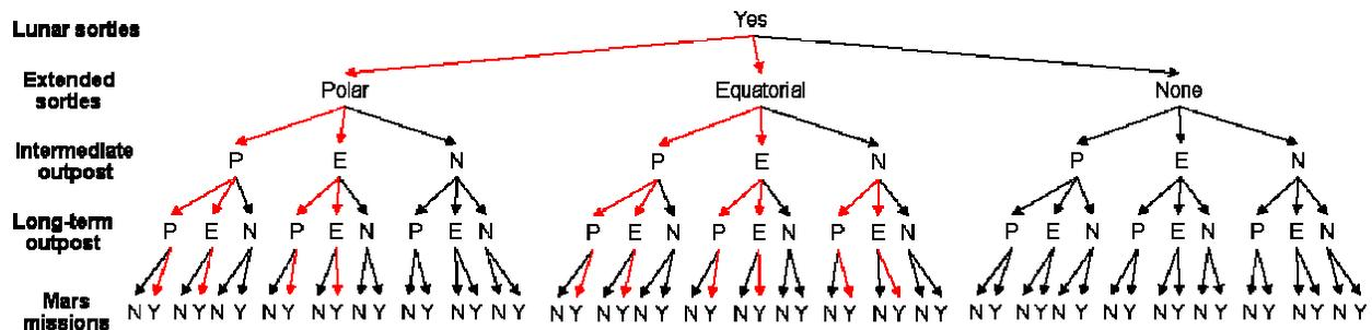
**Figure 3: Mission type scenarios for crewed Moon and Mars exploration capturing five different mission types. The four lunar mission types exhibit increasing levels of duration on the surface and of complexity; for Mars missions, conjunction class missions were assumed.**
