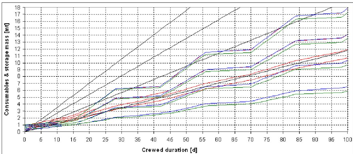
**Figure 9: Mass requirements for an equatorial intermediate outpost mission. Black lines represent baseline configuration (fuel cells, LiOH, no regeneration), red lines represent baseline configuration plus solar panels, blue lines represent red configuration plus wash water regeneration, green lines represent blue configuration plus regenerative CO2 removal. Contours represent different power levels, highest 20 kW, lowest 5 kW.**
