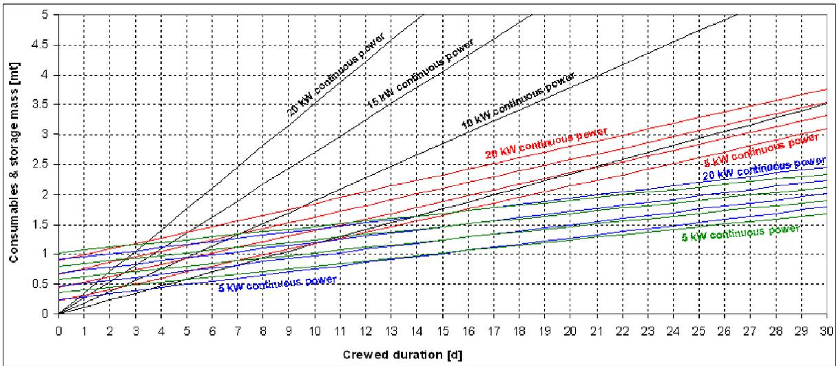
**Figure 4: Mass requirements for extending a polar sortie mission. Black lines represent baseline configuration (fuel cells, LiOH, no regeneration), red lines represent baseline configuration plus solar panels, blue lines represent red configuration plus wash water regeneration, green lines represent blue configuration plus regenerative CO<sub>2</sub> removal. Contours represent different power levels, highest 20 kW, lowest 5 kW.**
