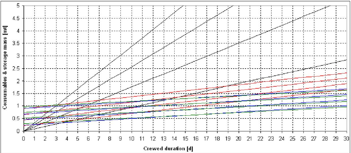
Figure 13: Mass requirements for extended polar LSAM stays of 2 crewmembers. Black lines represent baseline configuration (fuel cells, LiOH, no regeneration), red lines represent baseline configuration plus solar panels, blue lines represent red configuration plus wash water regeneration, green lines represent blue configuration plus regenerative CO<sub>2</sub> removal. Contours represent different power levels, highest 20 kW, lowest 5 kW.
