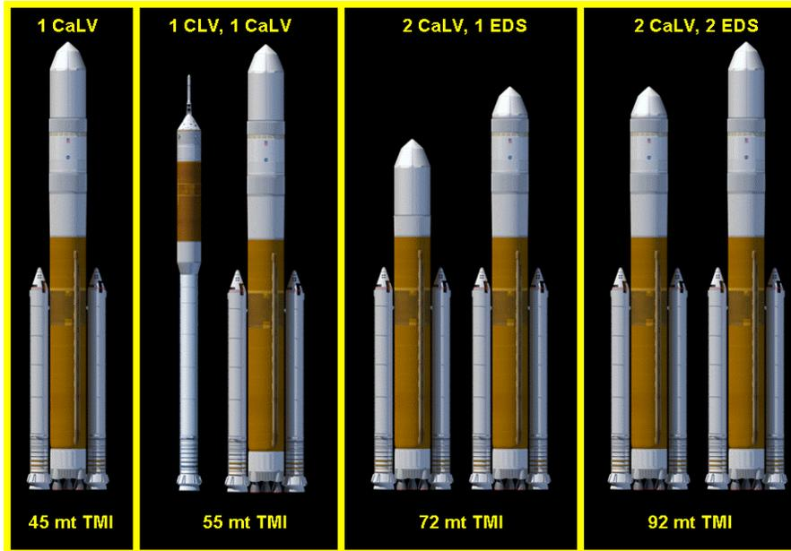
**Figure 10: Overview of ESAS CaLV and CLV derived Mars launch options showing Trans-Mars Injection (TMI) capability for 4,050 m/s burn from 400 km low Earth orbit. Dual launch options include rendezvous in Earth orbit prior to TMI.**
