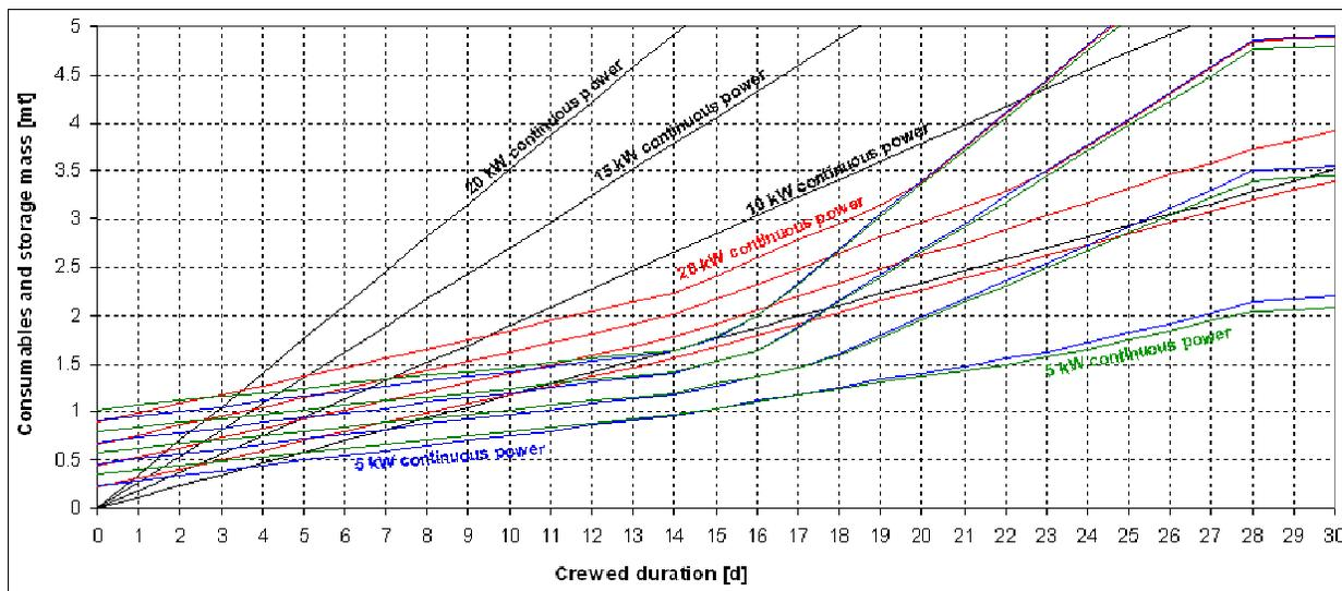
**Figure 5: Mass requirements for extending an equatorial sortie mission. Black lines represent baseline configuration (fuel cells, LiOH, no regeneration), red lines represent baseline configuration plus solar panels, blue lines represent red configuration plus wash water regeneration, green lines represent blue configuration plus regenerative CO<sub>2</sub> removal. Contours represent different power levels, highest 20 kW, lowest 5 kW.**
