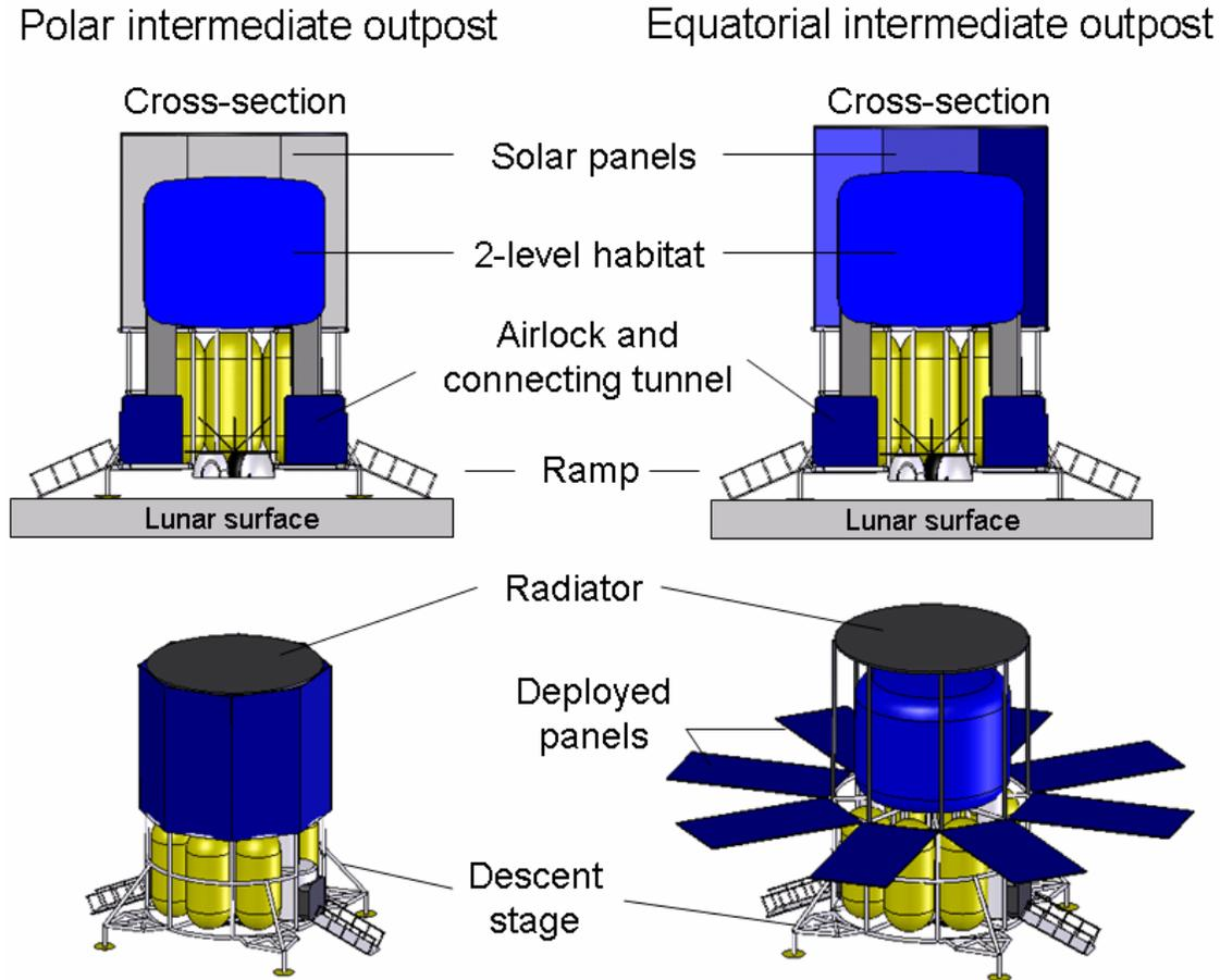
**Figure 2: Overview of the intermediate outpost reference design for polar and equatorial sites**
