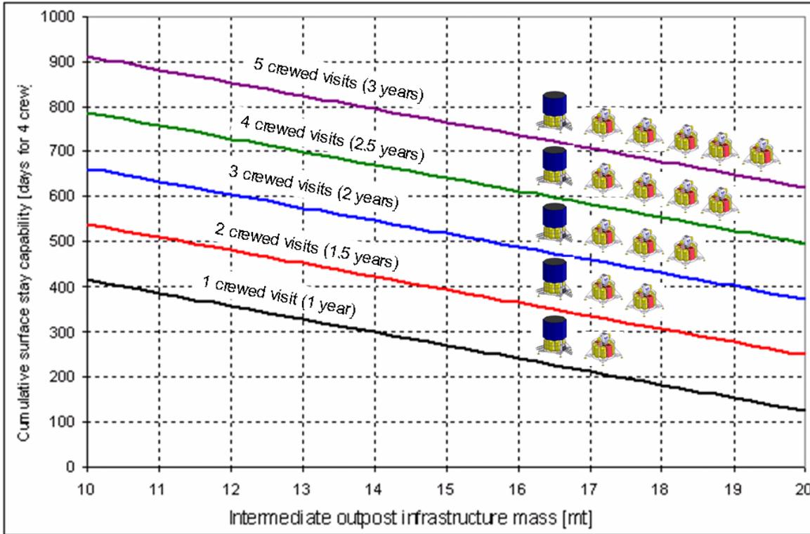
Figure 4: Cumulative surface crew time achievable as a function of intermediate outpost infrastructure mass and number of crewed visits to the intermediate outpost
