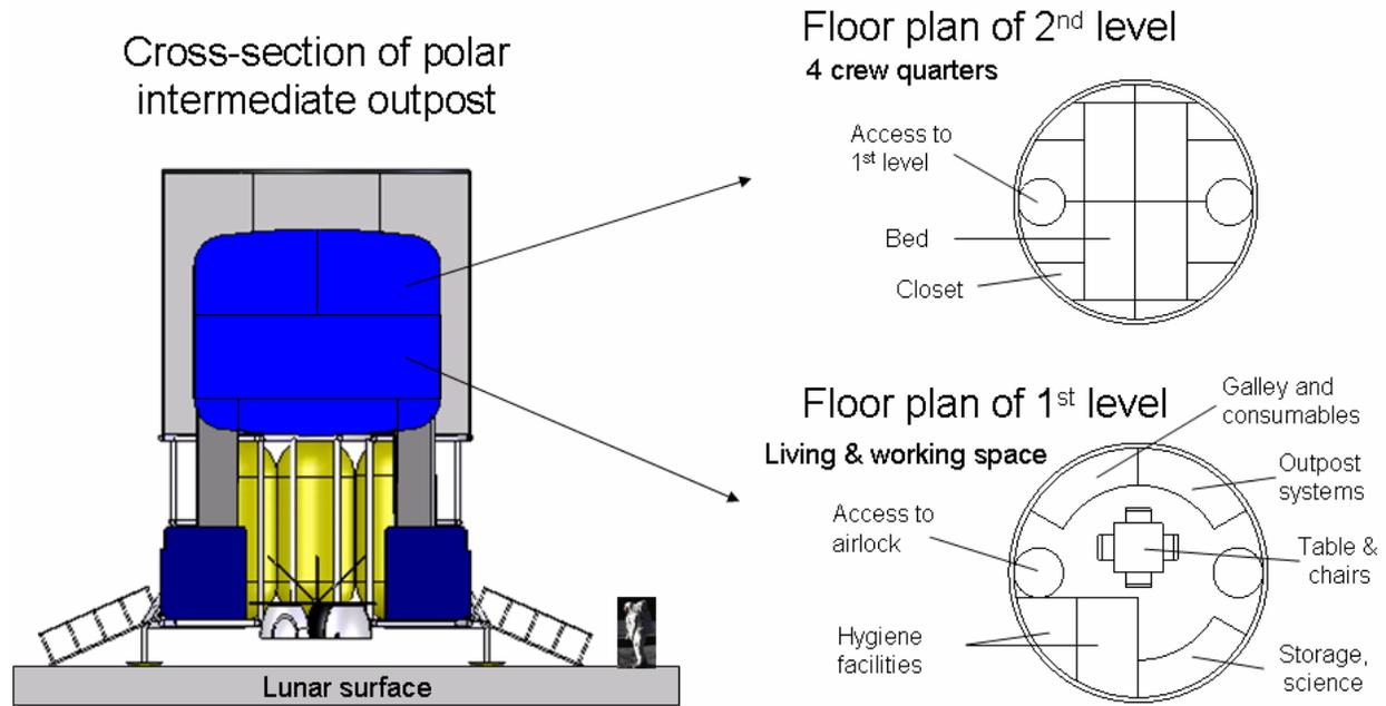
**Figure 3: Outpost habitat conceptual internal layout**
