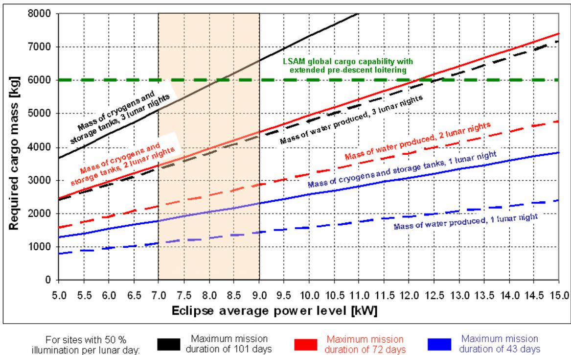
Figure 5: Cryogen storage requirements on LSAM for eclipse power generation at equatorial sites
