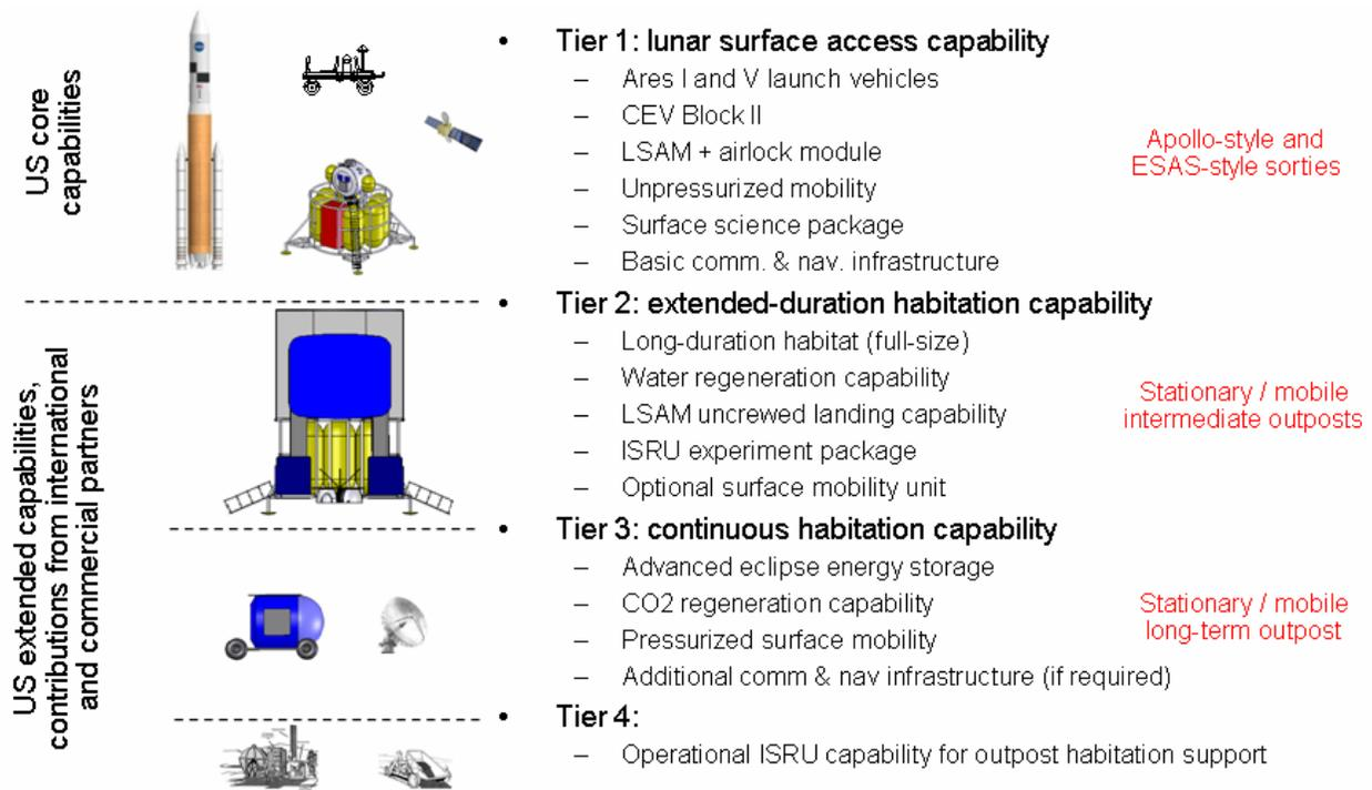
**Figure 17: Proposed development plan for lunar architecture elements in accordance with the assumptions of the Global Exploration Strategy (GES)<sup>1</sup>**
