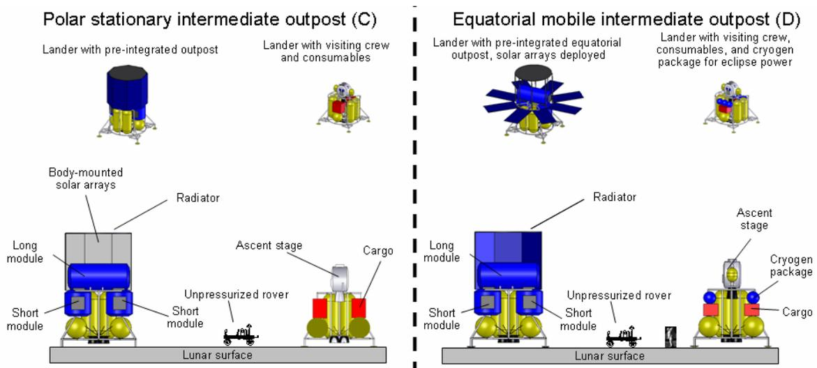
**Figure 5: Stationary and mobile intermediate outpost concepts based on small habitat modules**
