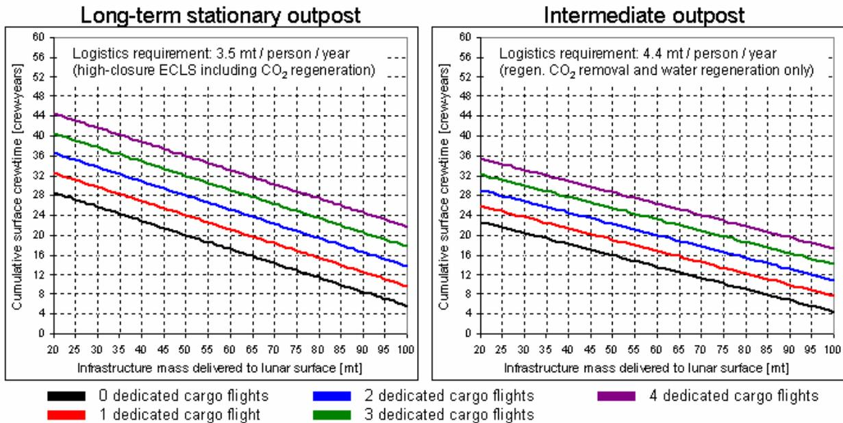
**Figure 10: Logistics diagrams for the long-term outpost (left) and intermediate outposts (right)**
