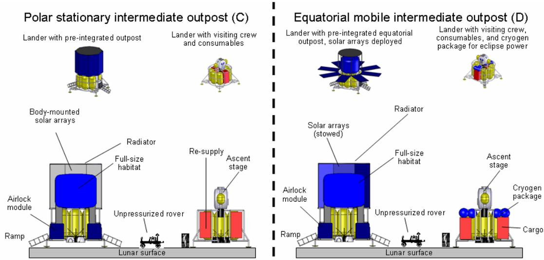
**Figure 8: Stationary and mobile intermediate outpost concepts based on full-size habitat module**
