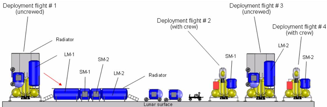
Figure 4: Stationary long-term outpost based on assembly of habitat modules
