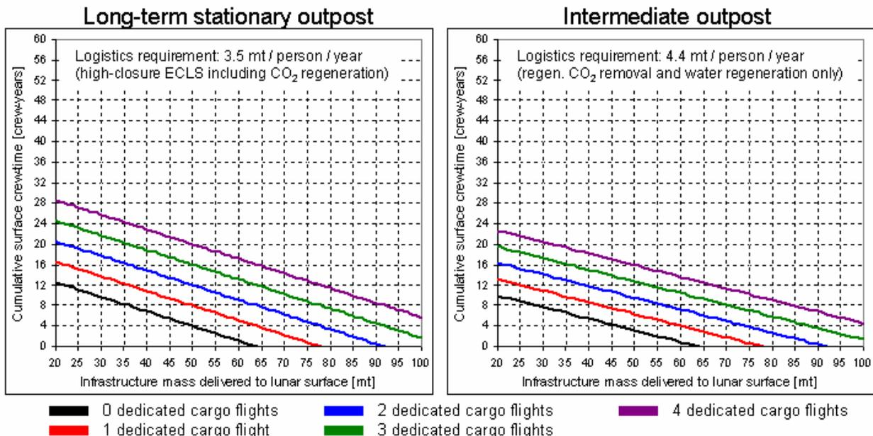
Figure 13: Logistics diagrams for degraded TLI capability
