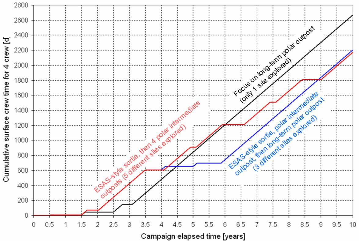
Figure 12: Comparison of example campaign performance for the Type 2 architecture
