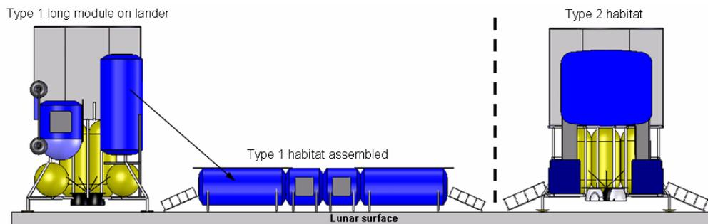
**Figure 15: Comparison of long-term outpost habitats for Type 1 and 2 architectures**
