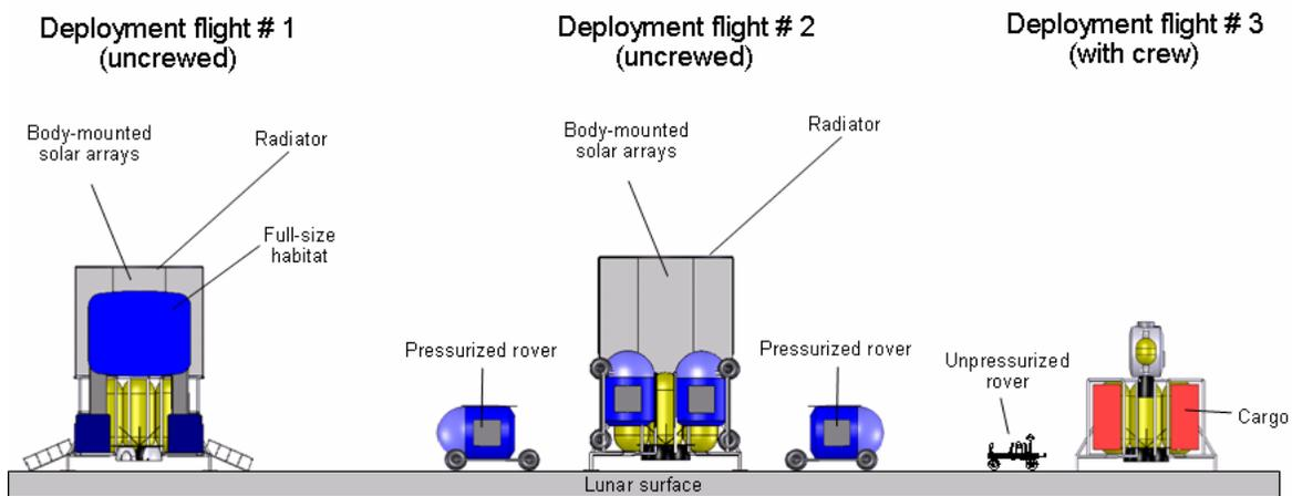
**Figure 7: Stationary long-term outpost based on pre-integrated full-size habitat module**
