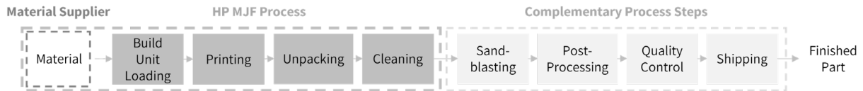
Figure 13. General additive manufacturing process using HP MJF technology.
