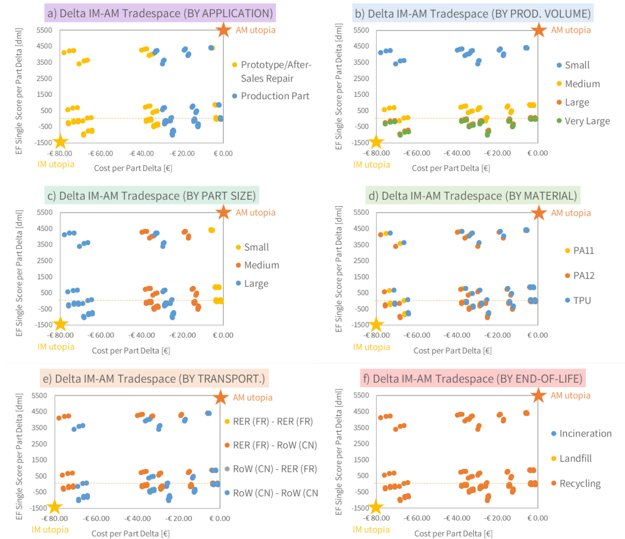
Figure 52. Tradespace graphs split by decision and showing EF and cost tradeoff between IM and AM.
